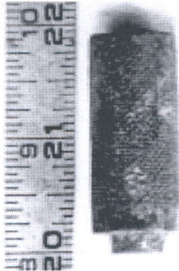
An unshielded caesium-137 found buried in gravel at a metal scrapyard in Illinois. The scale is in inches.
